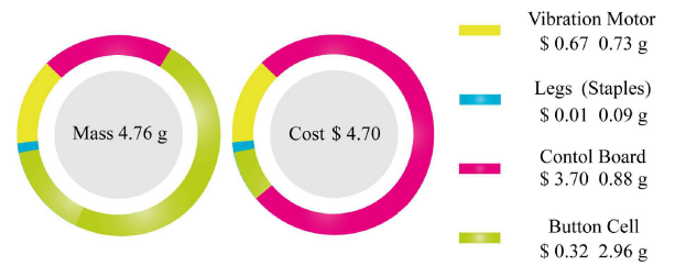
Fig. 9. Mass and cost contribution of each component of SimoBot.
