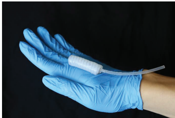
Fig. 1. The monolithic soft actuator made by the thermal casting method proposed in this work.
