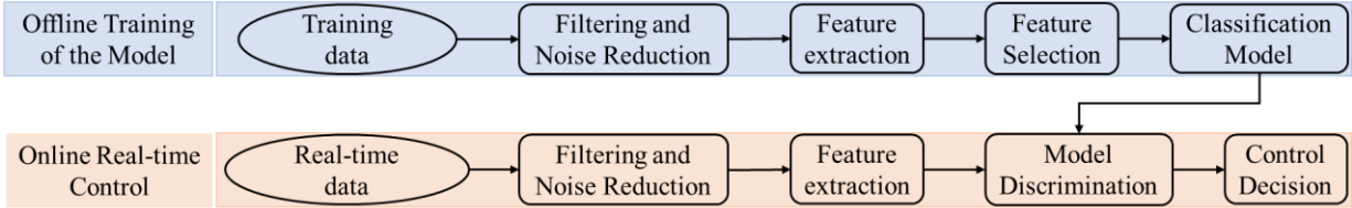
Figure S15. The flow chart of gesture recognition for a robot hand.
